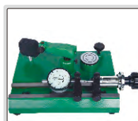
inspect accuracy of dial indicators (range 0-25mm)
