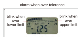
alarm when over tolerance
