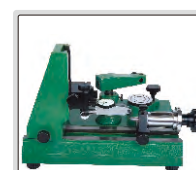
inspect accuracy of test indicators
