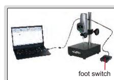
data transmitted to Excel without software
